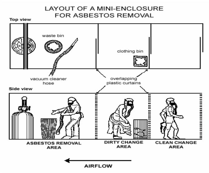
Figure 4 – Typical Layout of a Mini-Enclosure
