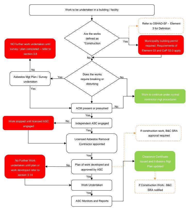
Figure 2 - Working with Asbestos
